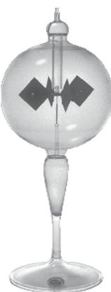
The Crookes radiometer is used for demonstrating the conversion of radiation energy into kinetic energy.
